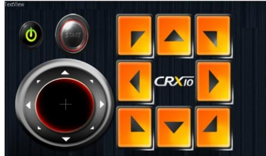
**Figure 4.** Track ball and Direction buttons for Remote Control of Mobile Robot
