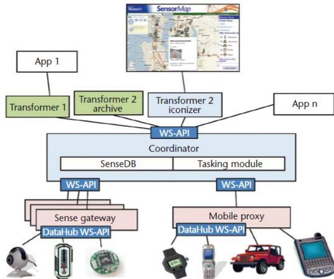
Figure 5. Microsoft SenseWeb: open system architecture for flexible sharing [16]
