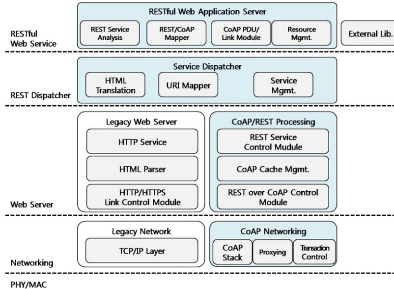
**Figure 7.** Software structure of WoT for BEMS
