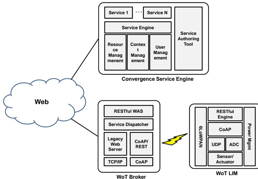
Figure 6. Overall architecture of WoT for BEMS
