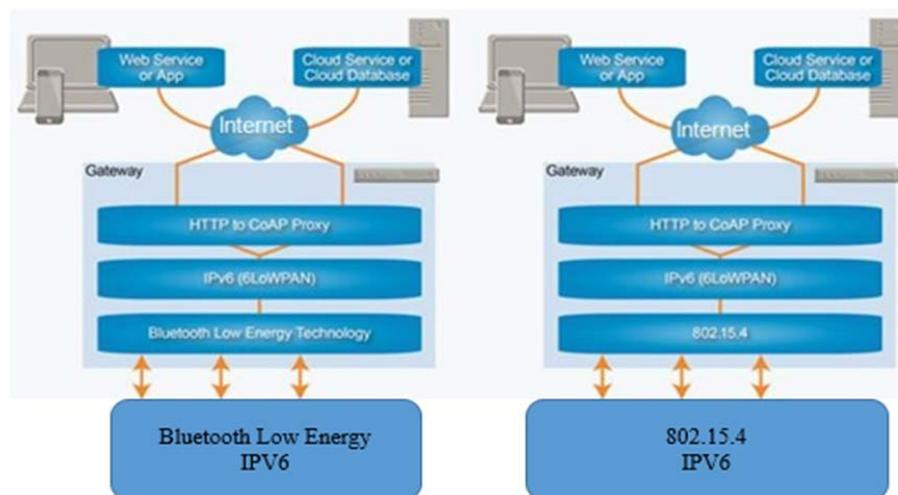
**Figure 8.** IP-based application in the sensor / device is transparently connected to an Internet [20]
