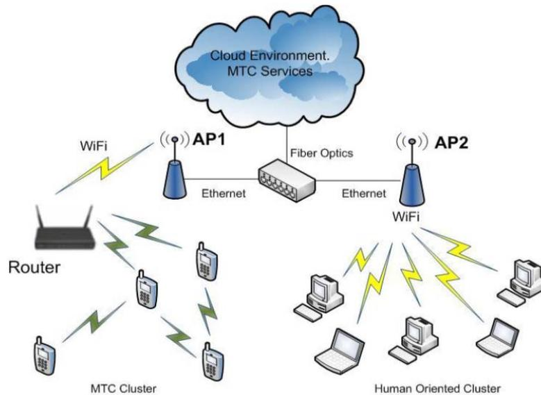
**Figure 7.** WLAN and IOT devices communication Architecture
