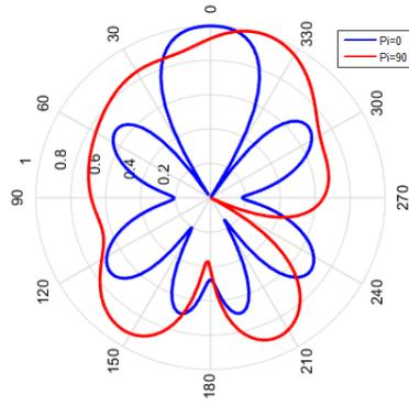
**Figure 10.** The normalized radiation patterns of  $2 \times 1$  array antenna
