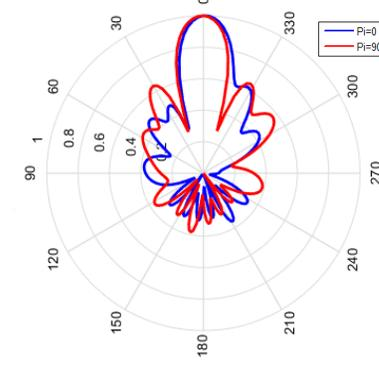
**Figure 13.** The normalized radiation patterns of  $4 \times 4$  array antenna
