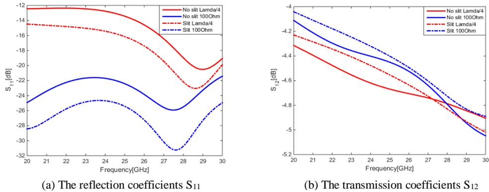
**Figure 6.** S Parametric plots for T-junction without/with slit.
