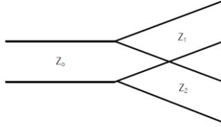
**Figure 1.** Transmission line model of a lossless T-junction
