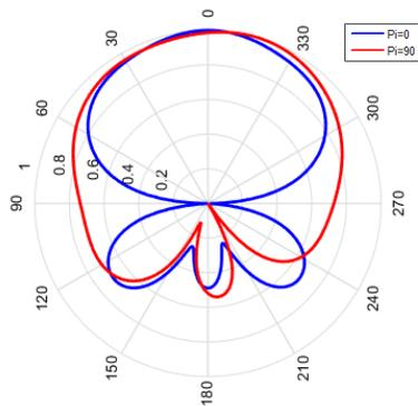
**Figure 8.** The radiation patterns of single patch antenna at 24 GHz
