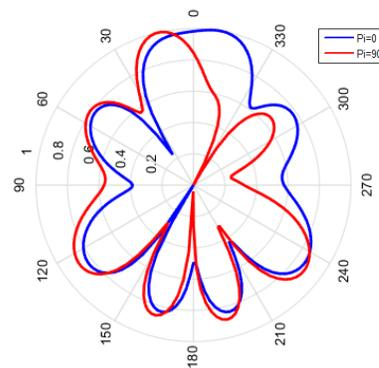
**Figure 11.** The normalized radiation patterns of  $2 \times 2$  array antenna
