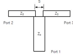
**Figure 3.** The inductive slit width  $S$  at the T-junction
