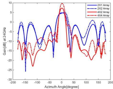
**Figure 9.** The comparison of simulated results on radiation pattern of array antennas
