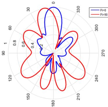
**Figure 12.** The normalized radiation patterns of  $4 \times 2$  array antenna
