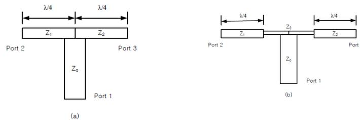
**Figure 2.** Designed T-junctions, (a)  $\lambda/4$ -transformer, (b)  $Z_3$  and  $\lambda/4$ -transformer
