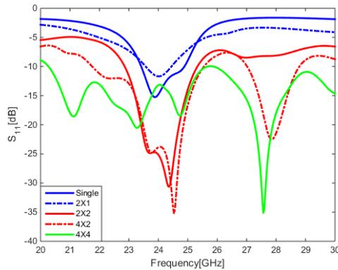
**Figure 7.** The reflection coefficient curves for the single patch,  $2 \times 1$  array,  $2 \times 2$  array,  $4 \times 2$  array, and  $4 \times 4$  array
