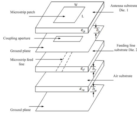
**Figure 4.** Aperture-coupled microstrip patch antenna
