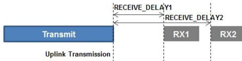
**Figure 5.** Data Transmission at the end-device of LoRaWAN
