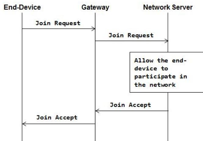
Figure 4. Join procedure of LoRaWAN
