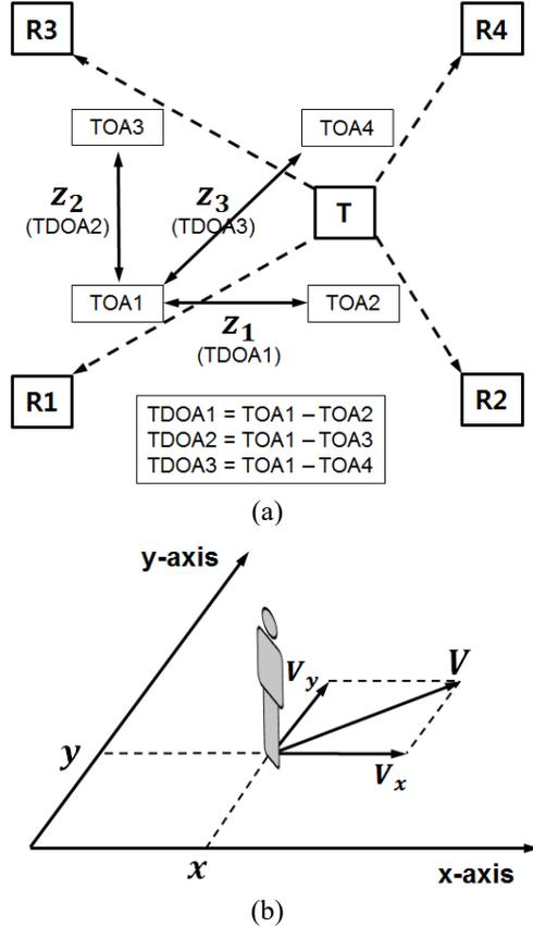
**Figure 1.** Human localization scheme: (a) TDOA measurements and (b) 2D geometry of human motion
