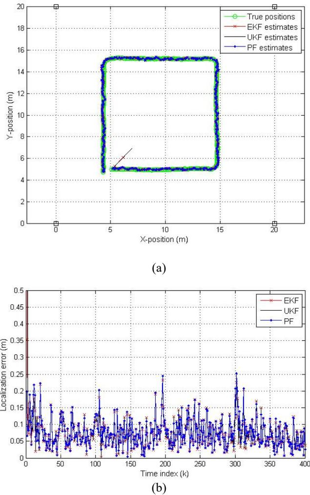
**Figure 3.** Localization results when  $\mathbf{Q}_k = 0.1^2 \mathbf{I}_4$ : (a) estimated positions by nonlinear filters, and (b) localization errors
