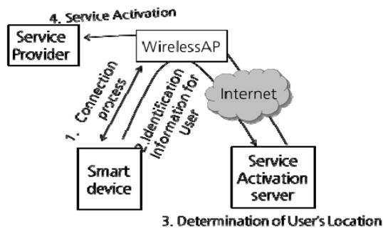
**Figure 1 .** Determination of users location by using information about wireless AP connection
