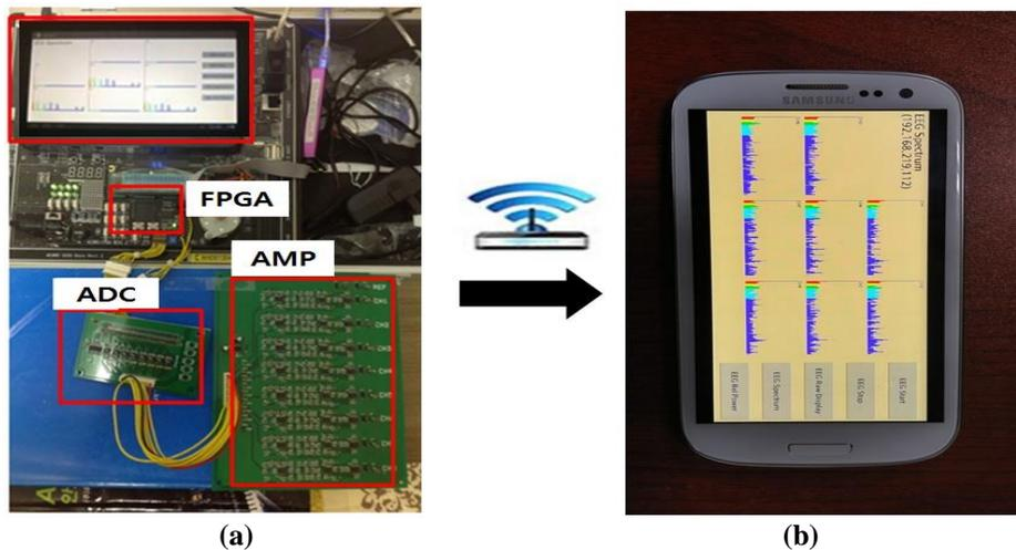
Figure 9. Entire system structure of the platform for EEG signal; (a) FPGA board; (b) smart phone
