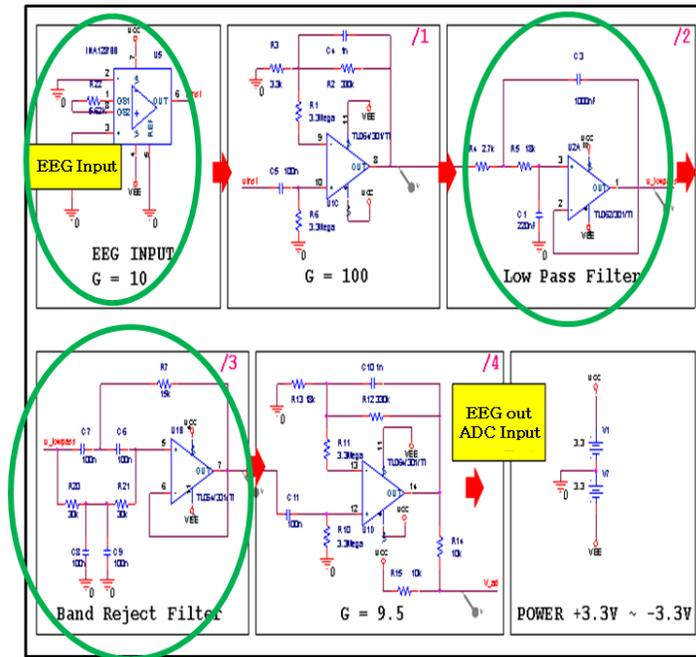
Figure 3. EEG sensor signal filter and amplifier circuit
