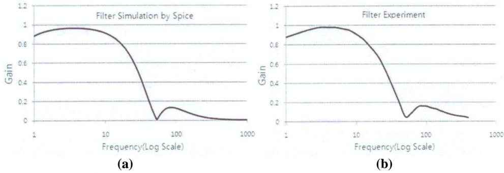
**Figure 5.** Results from (a) simulation and (b) actual experiment of the filter
