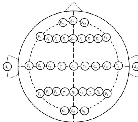
Figure 7. International 10-20 electrodes system
