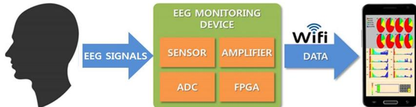
**Figure 2.** EEG monitoring system
