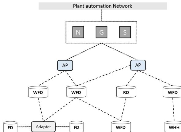
**Figure 4.** Network architecture of WirelessHART™ [13]
