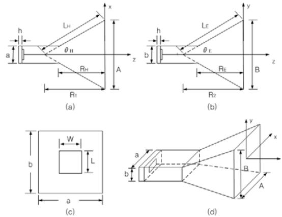
**Figure 1.** The microstrip patch-fed waveguide pyramidal horn antenna. (a) Cross section through the  $xz$ -plane, (b) Cross section through the  $yz$ -plane with the microstrip patch-fed, (c) The microstrip patch antenna (d) Overall geometry.
