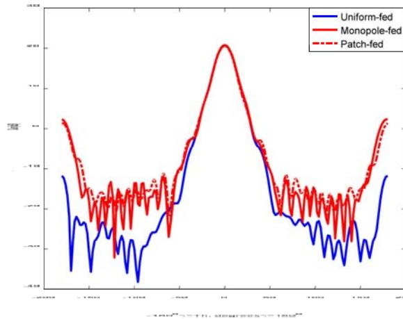
**Figure 5.** H-plane patterns of the pyramidal horn antenna with uniform-fed, monopole-fed, and patch-fed at 77 GHz.
