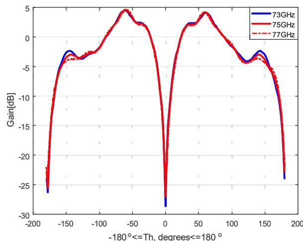
**Figure 3.** Radiation patterns of monopole antenna at the center frequencies of 73 GHz, 75 GHz, and 77 GHz.
