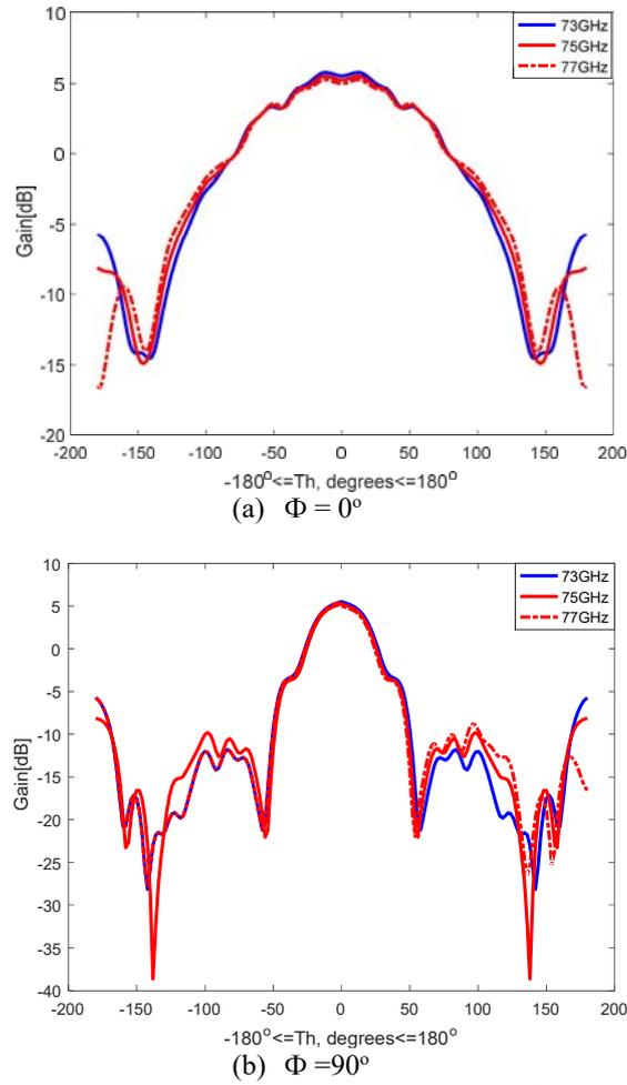
**Figure 4.** Radiation patterns of microstrip patch antenna at the center frequencies of 73 GHz, 75 GHz, and 77 GHz.
