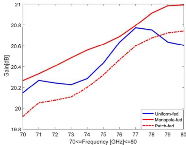
Figure 7. Gain characteristics of the pyramidal horn antenna with uniform fed and monopole fed.
