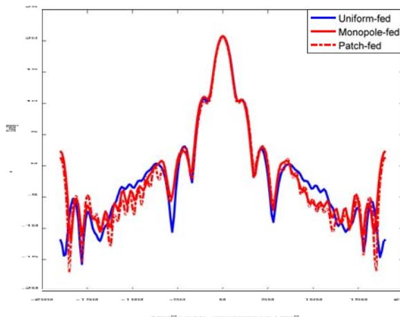
**Figure 6.** E-plane patterns of the pyramidal horn antenna with uniform-fed, monopole-fed, and patch-fed at 77 GHz.
