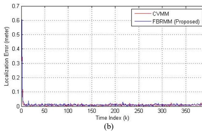
Fig. 3 MCL results when  $Q_k = 10^2 I_2$ : (a) real and estimated trajectory and (b) localization error.
