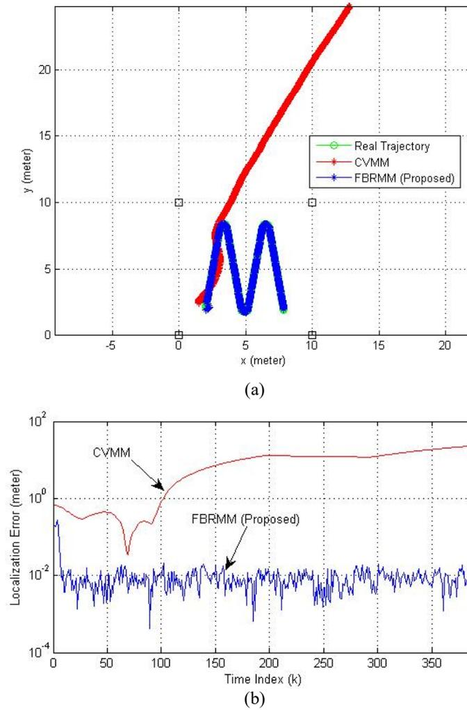
**Fig. 5** MCL results when  $\mathbf{Q}_k = 0.1^2 \mathbf{I}_2$ : (a) real and estimated trajectory and (b) localization error.
