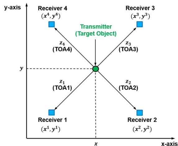
Fig. 1 2D schematic of wireless sensor network
