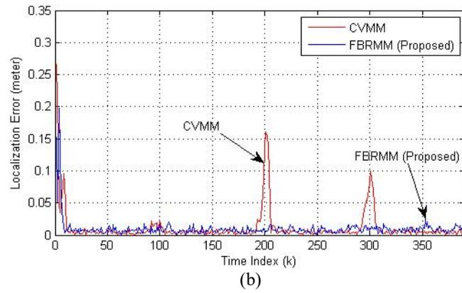
Fig. 2 MCL results when  $Q_k = I_2$ : (a) real and estimated trajectory and (b) localization error.
