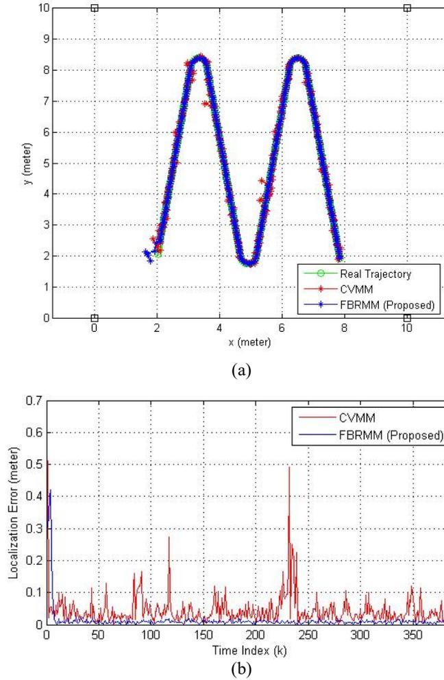
Fig. 4 MCL results when  $\mathbf{Q}_k = 50^2 \mathbf{I}_2$ : (a) real and estimated trajectory and (b) localization error.
