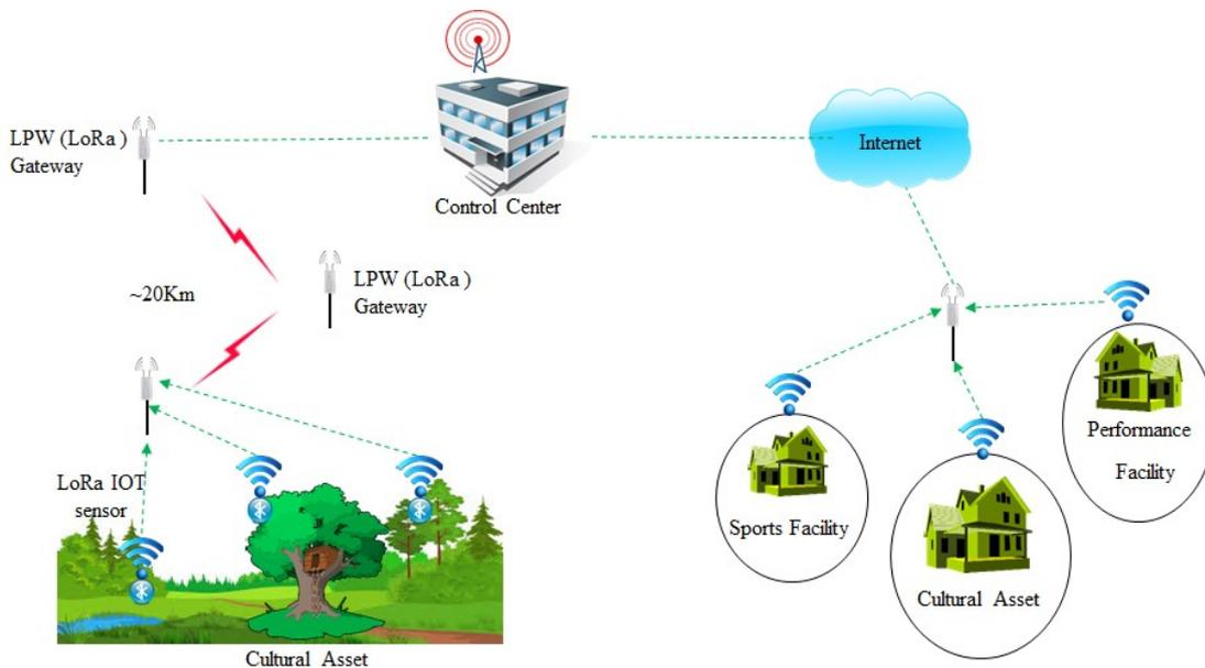
**Figure 1.** A Concept of Lora-based Real-time Cultural Facility Monitoring System.
