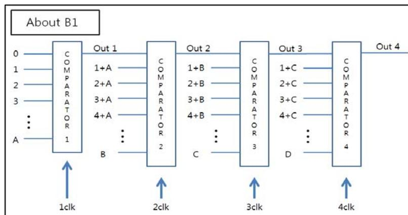
Figure 6. The structure of a four-stage pipeline comparator
